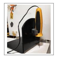
Set a 'Hot Wire Adjustable Sled Guide' and their 'Precision Engraver', to an appropriate depth. Slide across your foam surface, following the brick pattern.
